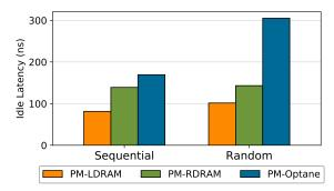
Figure 7: **Read latency** An experiment showing random and sequential read latency to Optane DC memory on a cache miss. Optane DC memory is about  $3 \times$  slower than DRAM for random accesses and about  $2 \times$  slower for sequential access (see data in csvroot/basic/idle\_latency.csv).
