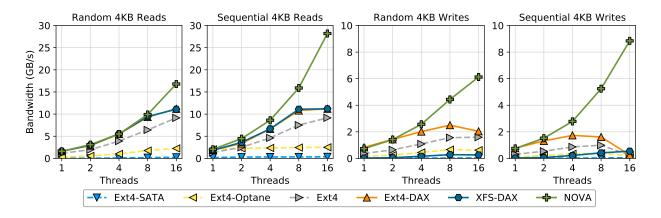
Figure 5: **Raw Performance in Persistent Memory File Systems** Optane DC PMMs provides a big boost for basic file access performance compared to SATA SSDs ("Ext4-SATA") and Optane-based SSDs ("Ext4-Optane"). The data also show the improved scalability that NOVA offers relative to legacy file systems in DAX mode.
