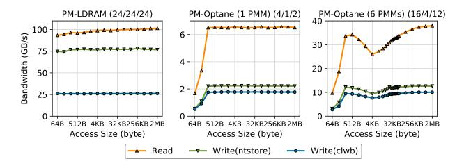
Figure 11: **Bandwidth over access size** An experiment showing maximal bandwidth over different access sizes on (from left to right) local DRAM, on a single Optane DC PMM, and interleaved Optane DC memory across six Optane DC PMMs. Graph titles include the number of threads used in each experiment (Read/Write(ntstore)/Write(clwb)) (see data in csvroot/basic/bw\_access\_size\_dram.csv, csvroot/basic/bw\_access\_size\_optane\_1pmm.csv and csvroot/basic/bw\_access\_size\_optane\_6pmms.csv).
