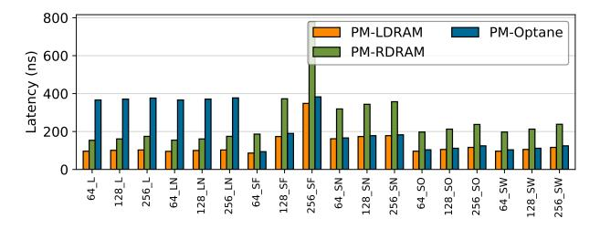
Figure 8: **Memory Instruction Latency** This graph shows the median latency for a variety of ways of accessing persistent memory. Note that for store instructions followed by flushes, there is little performance difference between PM-LDRAM and PM-Optane, whereas DRAM outperforms Optane DC memory for load sequences (see data in csvroot/basic/instruction\_latency.csv).
