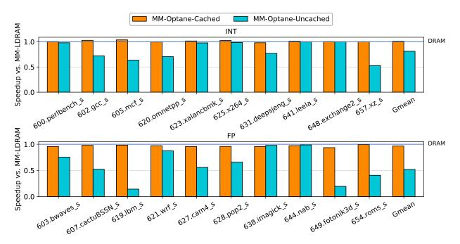
Figure 3: **SPEC 2017 Performance on Optane DC** Using cached Optane DC instead of normal DRAM does not affect performance for the integer workloads in SPEC 2017. Without caching, performance drops 38%. For floating point, cached Optane DC drops performance for the floating point workloads by 15%, probably due to bandwidth limitations. Uncached drops it by 61%.
