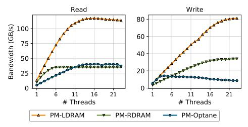
Figure 1: **Optane DC Sequential Bandwidth** The data show read (left) and write (right) bandwidth for an array of six Optane DC PMMs compared to a similar array of six DRAM DIMMs. Optane DC bandwidth is lower and, for writes, reaches saturation with fewer threads.
