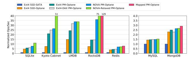
Figure 6: **Application Performance on Optane DC and SSDs** These data show the impact of more aggressively integrating Optane DC into the storage system. Replacing flash memory with Optane DC in the SSD gives a significant boost, but for most applications deeper integration with hardware (i.e., putting the Optane DC on a DIMM rather than an SSD) and software (i.e., using an PMEM-optimized file system or rewriting the application to use memory-mapped Optane DC) yields the highest performance.
