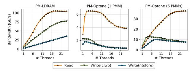
Figure 10: **Bandwidth vs. thread count** An experiment showing maximal bandwidth as thread count increases (from left to right) on local DRAM, on a single Optane DC PMM, and interleaved Optane DC memory across six Optane DC PMMs. All threads use a 256 B access size. (Note the difference in vertical scales). (see data in csvroot/basic/bandwidth\_dram.csv, csvroot/basic/bandwidth\_optane\_1pmm.csv and csvroot/basic/bandwidth\_optane\_6pmms.csv)
