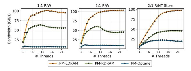
Figure 12: **Sequential memory bandwidth with different # threads for mixed workloads** This graph shows memory performance under a varying number of threads performing (from left to right) reads and writes with 1:1 ratio, reads and writes with 2:1 ratio, or reads and non-temporal stores with 2:1 ratio (see data in csvroot/basic/mixed\_bandwidth\_1r1w.csv, csvroot/basic/mixed\_bandwidth\_2r1w.csv and csvroot/basic/mixed\_bandwidth\_2r1nt.csv).
