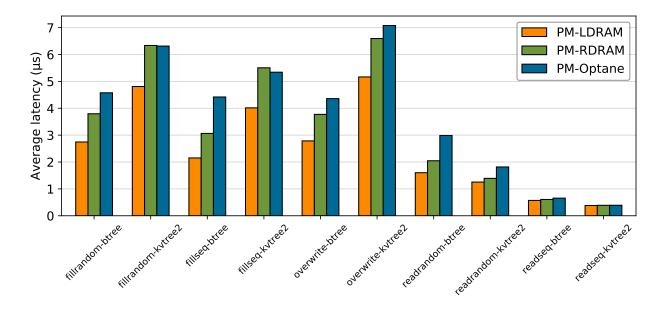
Figure 36: **Implications of Optane DC on Intel's PMemKV performance**: We report average latency of performing random insert, sequential insert, random read, sequential read and overwrite operations against PMemKV's storage engines (btree and kvtree2). Compared to PM-LDRAM, running PMemKV on PM-Optane shows similar latency for sequential read but up to  $2.05 \times$  higher latency for write operations (see data in csvroot/pmem/pmemkv.csv).
